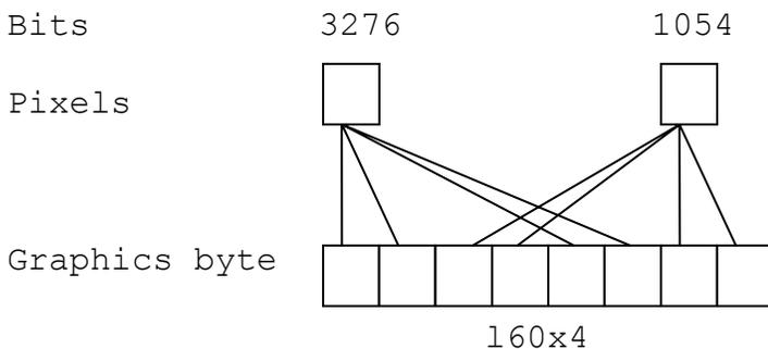
320A mode is a direct mapping, like 160x2, except that each bit specifies the color of one pixel.
